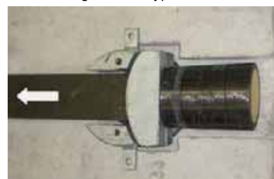
III. 3: ancrage fixe type III
